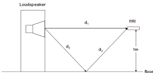
Fig 1 Floor reflection geometry
