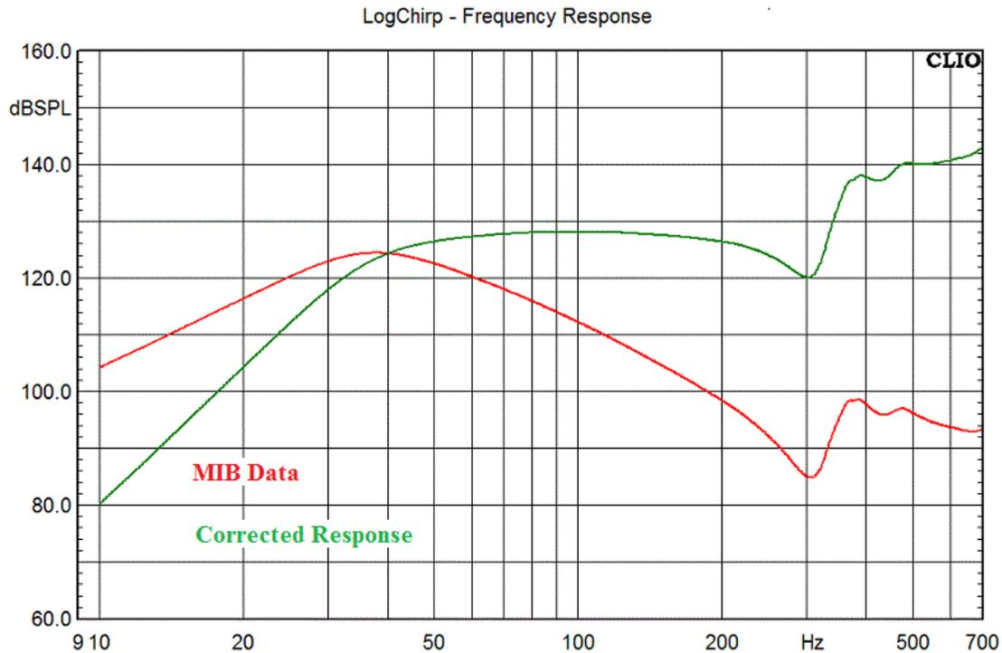
**Fig 7 Two-way MIB measurements**
