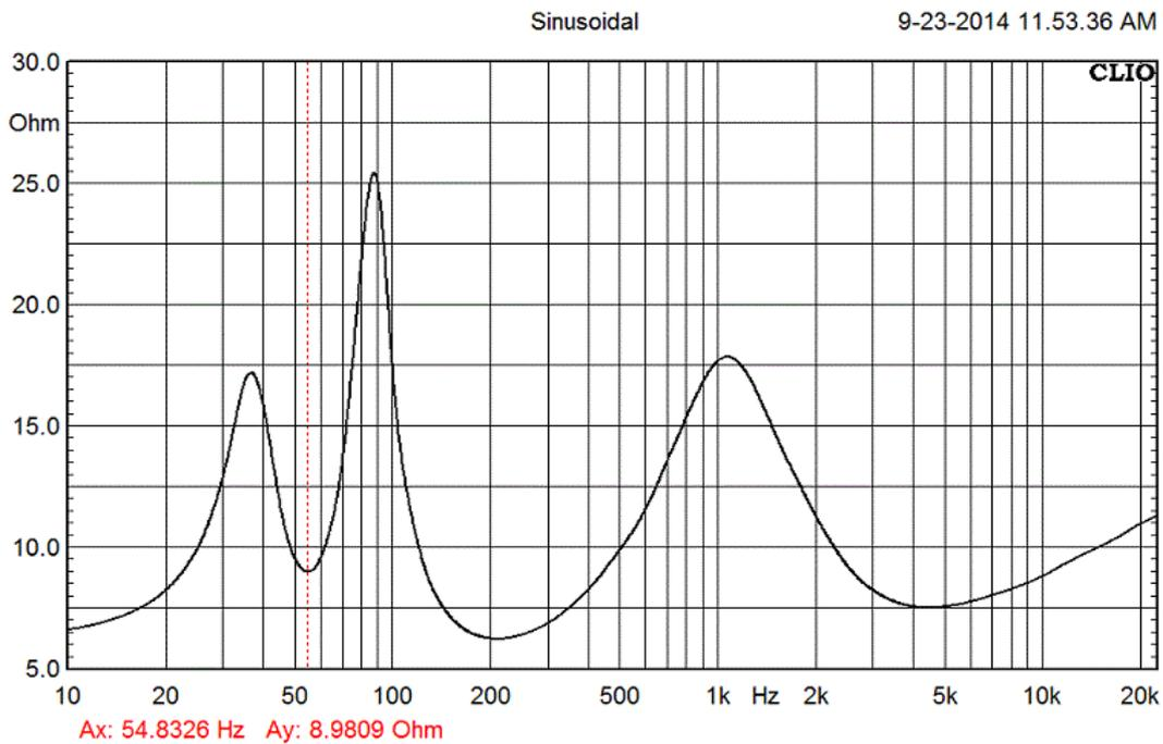
**Fig 14 Small Two-Way Impedance Plot**
