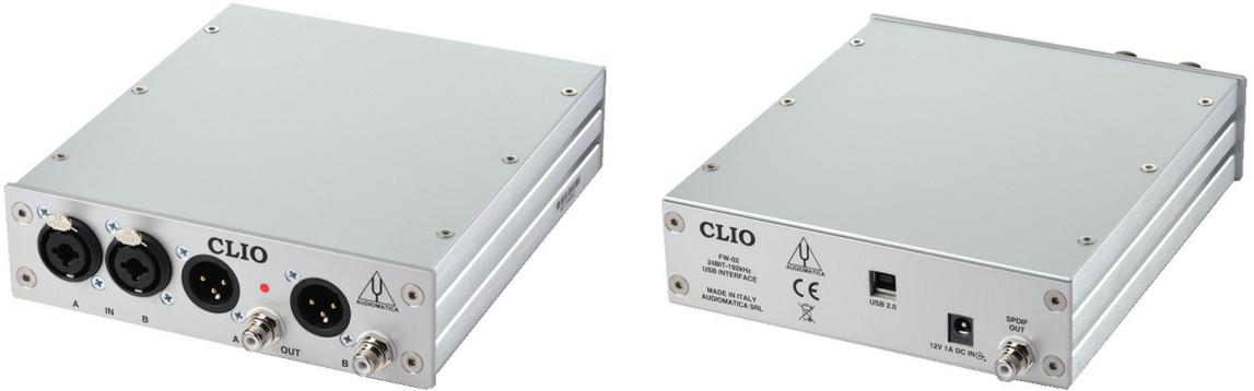
This unit is needed to correctly interface analog signals to your PC; it is also important as it has an internal reference used to calibrate the system and also stores the system's serial number inside its internal EEPROM; Figure below shows where is located your CLIO system serial number.
