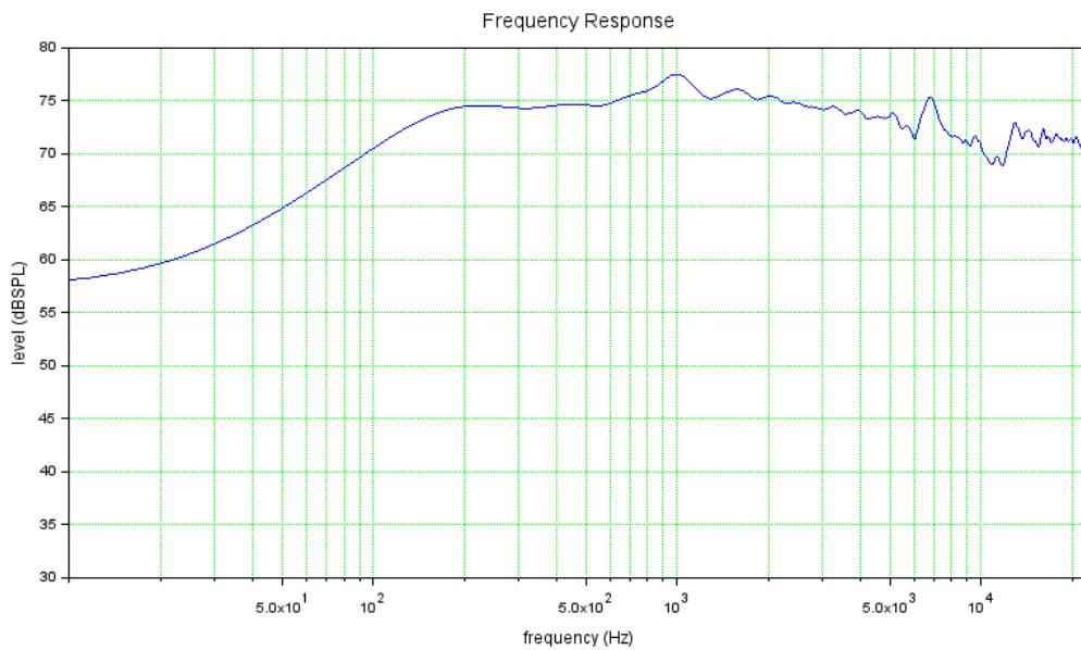
Please note that we are limiting the plot of our vectors in the range from index 2 to **MLSsize**/2 since we are interested only on the FFT positive frequency axis and we would avoid DC (zero frequency) to plot on a log-scale frequency graph. We also applied a +94 dB factor because measurements are in dB SPL referenced to 20 uPa.
