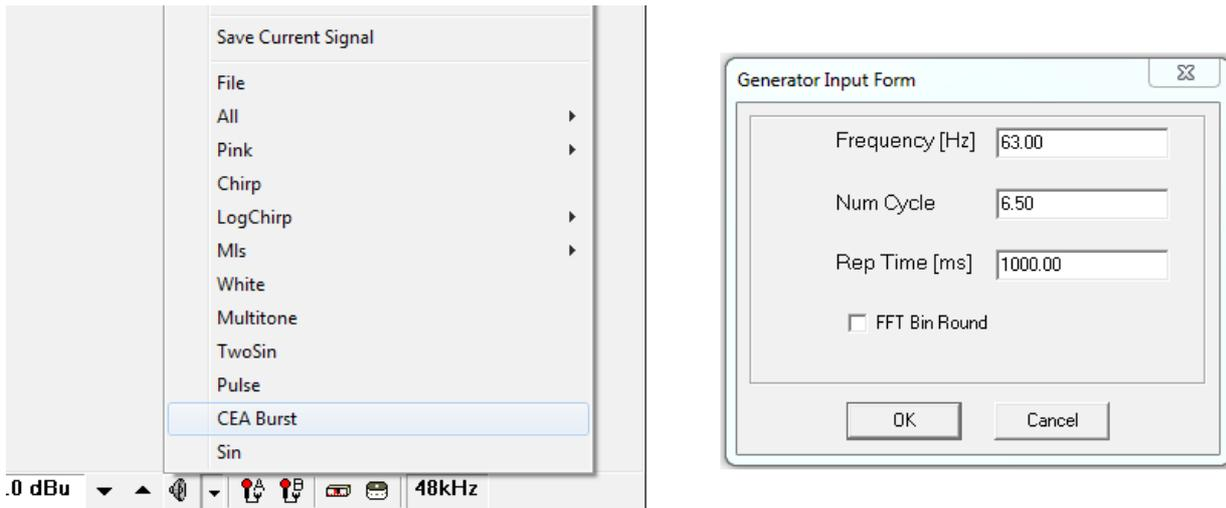
Figure 4: CEA Burst generator option and dialog
