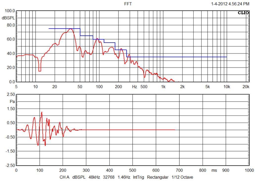
Figure 11: ACE-bass B2-50 - ANSI/CEA-2010 test @ 31.5 Hz
