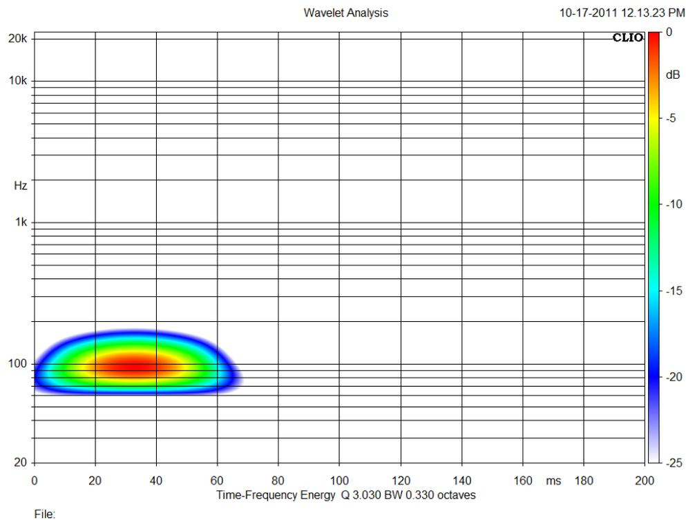
Figure 2: Joint time-frequency analysis (wavelet) of a 6.5 cycles 100 Hz hann-burst
