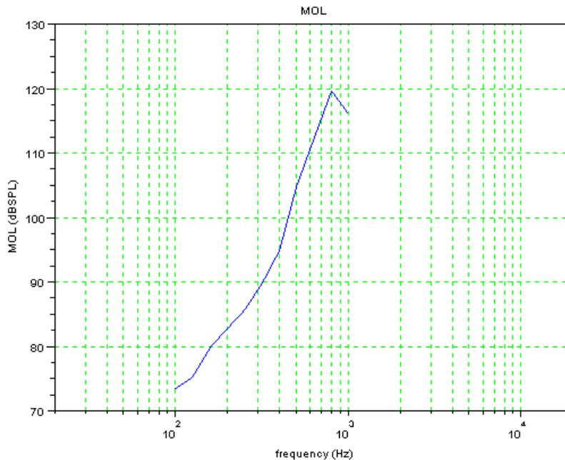
The above picture shows the MOL of a loudspeaker with THD>1.5%.
