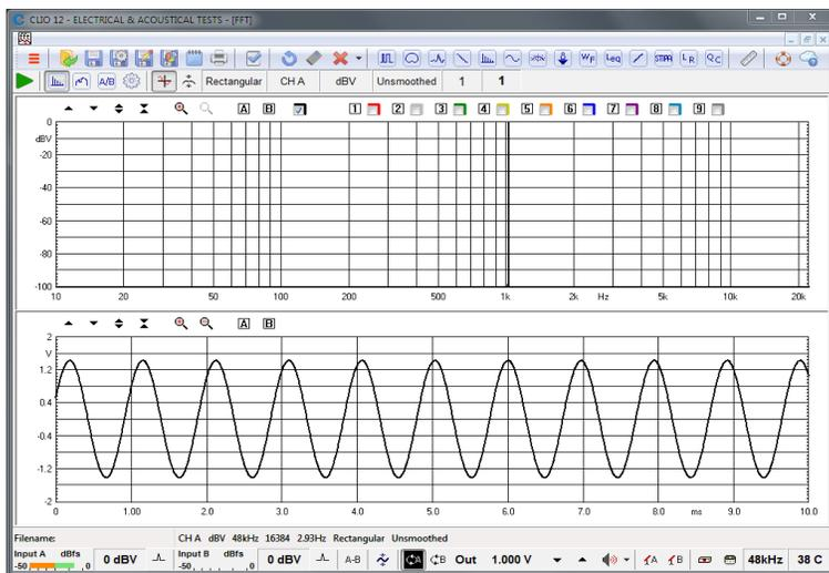
The result you should obtain is an FFT analysis of the 1kHz sinusoid (one spectral line @ 1kHz at 0dBV) and its time representation given by its oscillogram.
