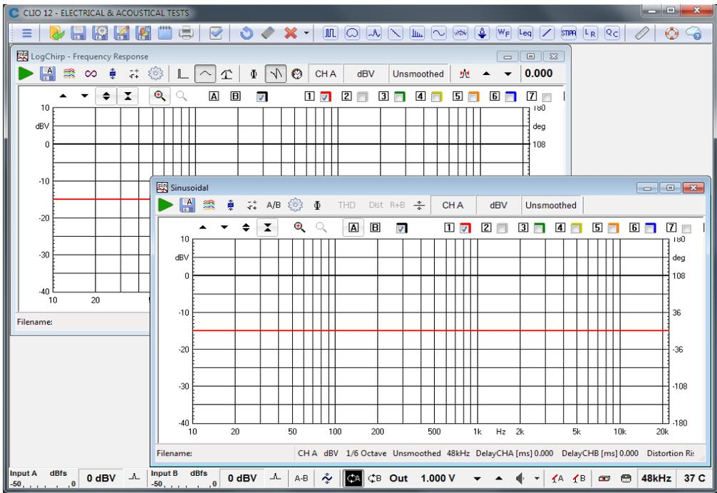
To ensure a 100% correct calibration you also need to inspect the phase responses of both measurements. To do this press the phase button  $\Phi$  and verify that you obtain a straight line (red curves) the readings in this case should be around zero degrees in both cases.
