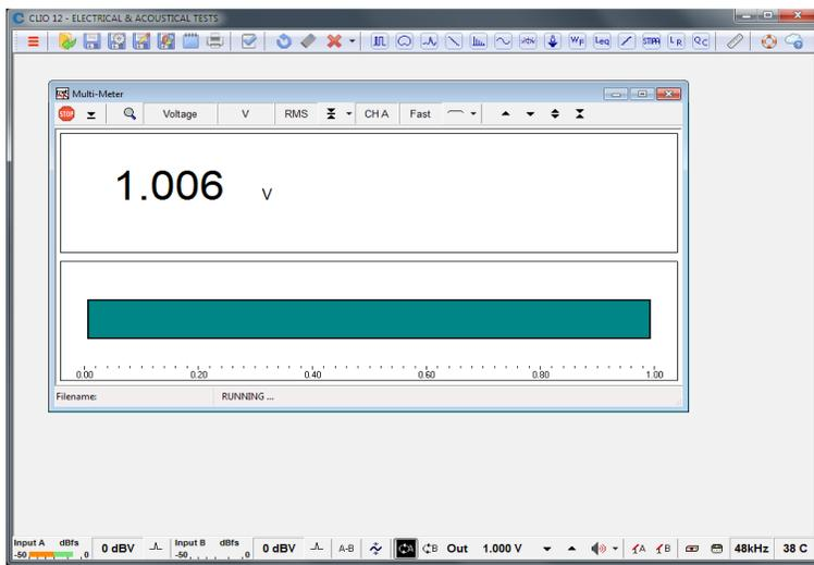
If everything is OK you should obtain a reading of circa 1V, variable between a minimum of 0.95V and a maximum of 1.05V, which is the mean output level of a sinusoidal signal when the system is not calibrated.
