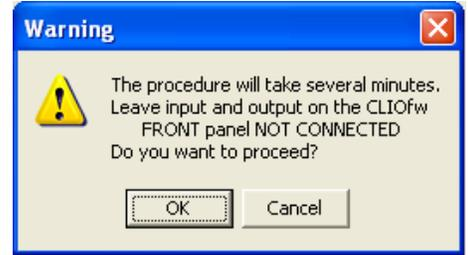
Answer **OK** to the initial prompt; this will run an automatic procedure that will last several minutes. The calibration procedure is completely automatic and several progress indicators will accompany all the executed measurements. At the end of it your CLIO system should be calibrated and ready to carry out measurements.
