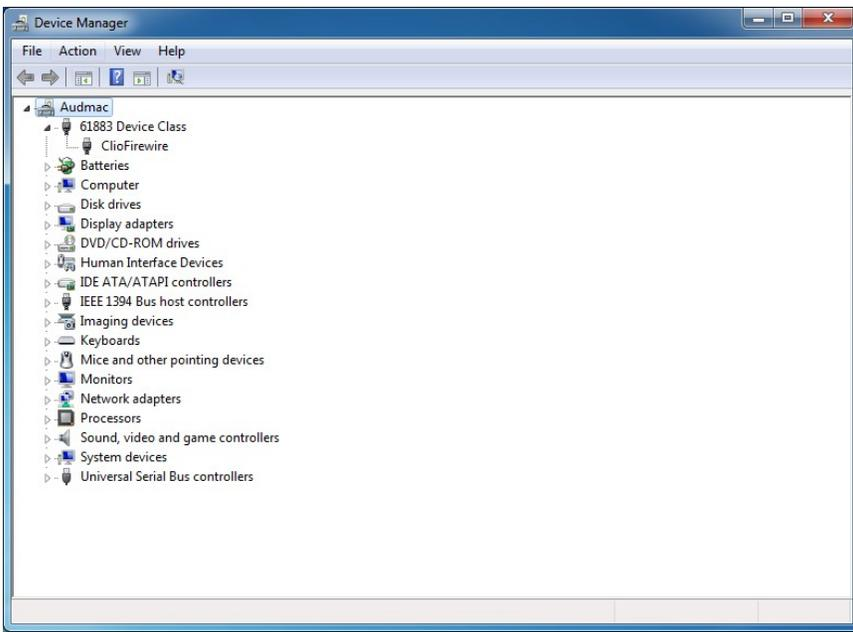
Verify the presence of the 'Clio Firewire' driver under the 61883 device class.
