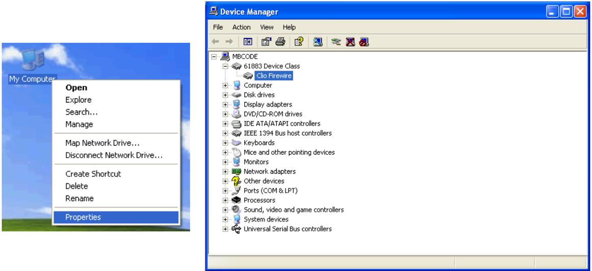
Verify the presence of the 'Clio Firewire' driver under the 61883 device class.
